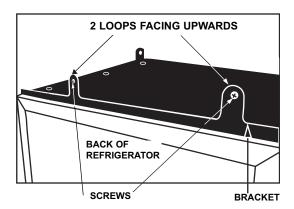
2. With the bracket lined up as stated above the preset holes on top of the refrigerator should be lined up with the holes on the bracket. Attach the bracket to the refrigerator using the six screws that come supplied with the refrigerator.
