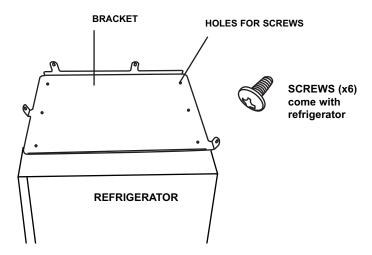
3. Place the microwave oven on top of the refrigerator and inside the two upright loops on the sides and in front of the two upright loops on the back of the bracket. Line up the holes on each side and on the back of the bracket and attach the microwave using the screws supplied. The two back screws come supplied with the refrigerator while the two side screws are already on the microwave. Please remove the two microwave screws prior to placing the microwave oven on top of the refrigerator.
