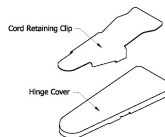
2. Slide Cord Retaining Clip to Hinge Cover until it stops.
