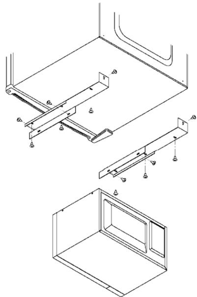
5. Place the left bracket flush with the top left side of the refrigerator/freezer with its rear lip facing downward over the back edge of the refrigerator/freezer, the shorter bend without holes should face outward.
